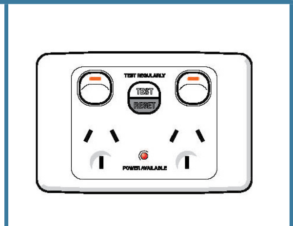
FIGURE 2: Fixed socket outlet RCD unit
