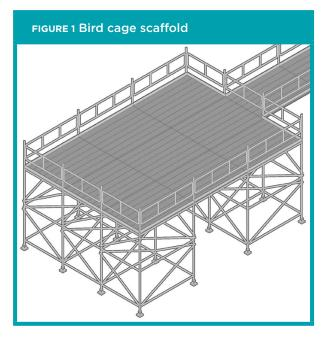
A fall arrest system is generally not a suitable risk control measure for the erection or dismantling of perimeter and birdcage scaffolds. You should refer to the <u>General guide for</u> <u>scaffolds and scaffolding work</u> for further information on fall arrest systems.
