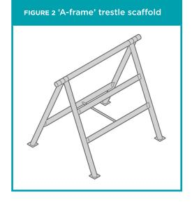
A trestle scaffold should be stable and erected on a suitable foundation to ensure it can safely
