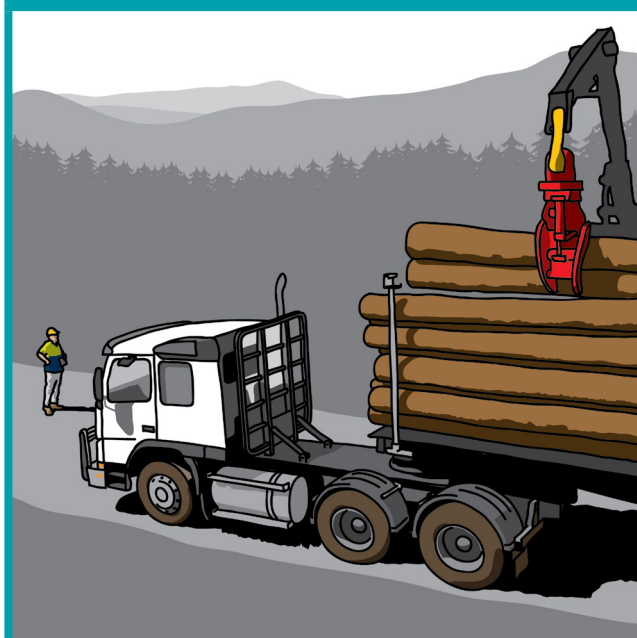
FIGURE 2 Example of a designated safe work position for a truck driver during loading
