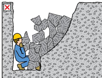
(c) Worker trapped and crushed against the trench wall by the quick collapse.
