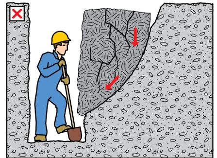
(b) Shear plane failure along the seepage (slippage) plane.
