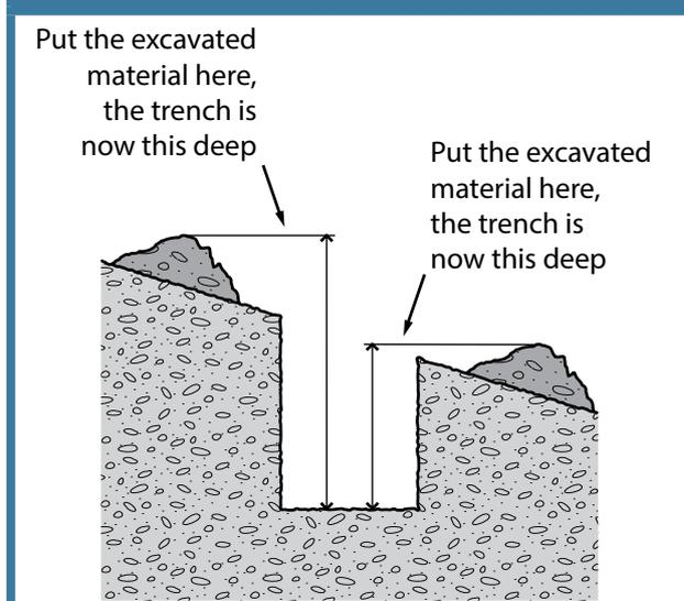
Care should be taken to ensure that material placed on the high side of the excavation does not increase the risk of ground collapse, or flooding by ponding or holding back runoff water. Excavated material should be placed so that it channels rainwater and other run-off water away from the excavation.
