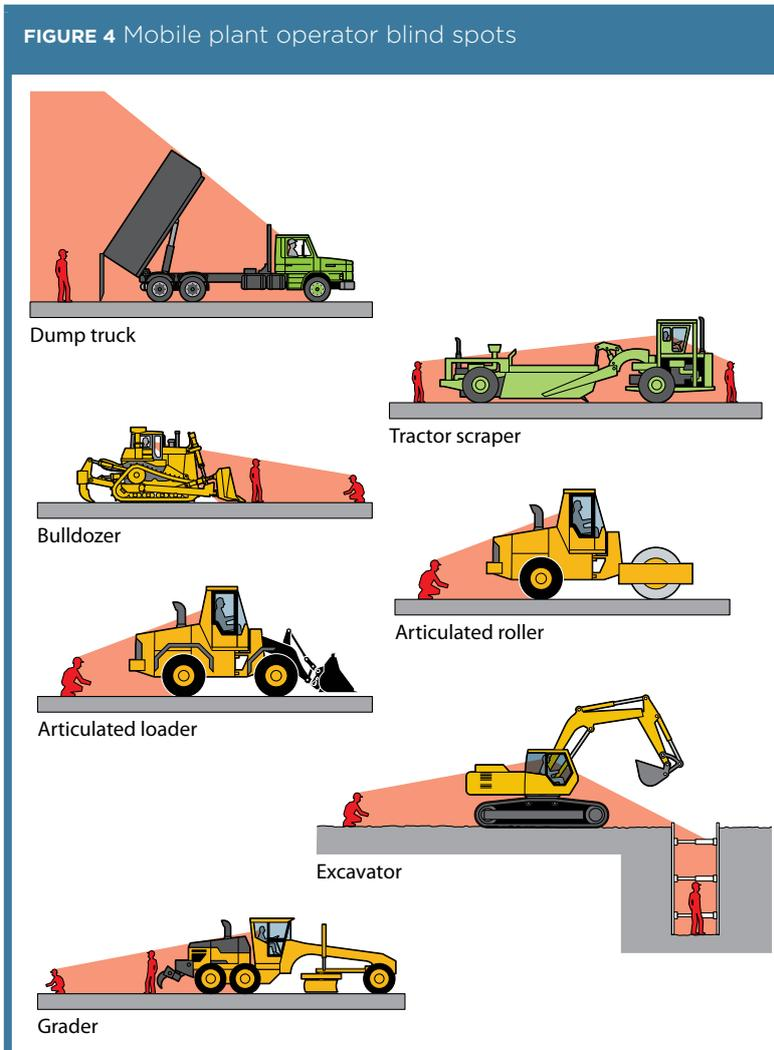
Powered mobile plant operating near ground personnel or other powered mobile plant should be equipped with warning devices (for example reversing alarm and a revolving light).
