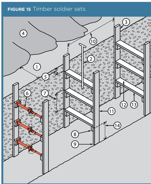
1. Spoil heap at least 1000mm clear of excavation allows access along the side of the trench top and prevents material from the heap rolling into the trench.
