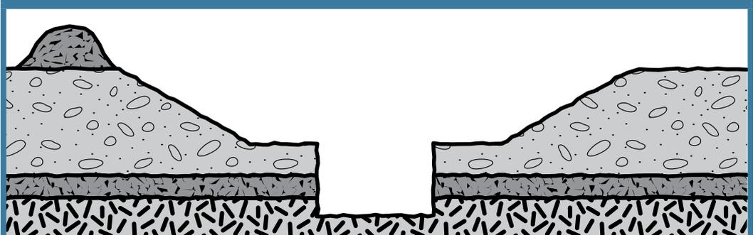
Benching and battering of excavation walls can minimise the risk of soil or rock slipping onto the excavation. Control measures should be designed by a competent person (for example geotechnical engineer) and be relative to the soil type, the moisture content of the soil, the planned height of the excavated face and any surcharge loads acting on the excavated face.
