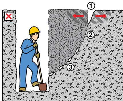
(a) This is a very dangerous situation, requiring ground support. No worker should be in the trench > 1.5m deep unless support has been installed.
