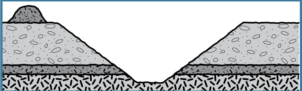
FIGURE 11 Combination of benching and battering controls
