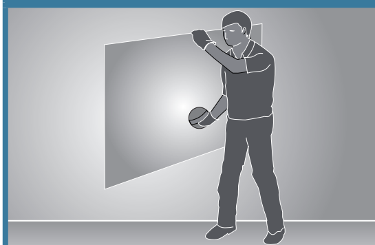
FIGURE 26 Use handling grip devices adapted to the particular object to be carried.
