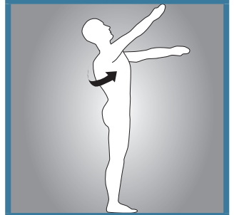
FIGURE 14 Bending the back or head backwards more than 5 degrees or looking up
